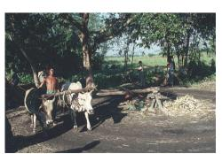
Figure 1: Animal powered crusher. Photo: Neil Cooper/Practical Action.
